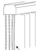
**! WARNING:** Do not traverse the blind with the vanes in the closed position.
