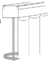
**Chain Control:** Pull the chain once in each direction, rotating the vanes open and closed.
