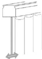
**Chain Control:** Pull the cord to ensure the blind traverses smoothly in both directions.
