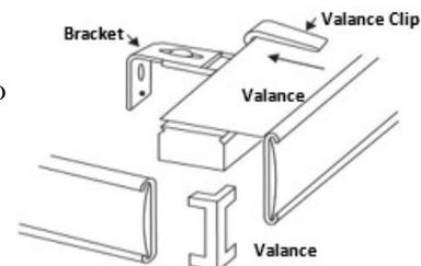
Valance returns may be trimmed to fit using heavy duty scissors.
